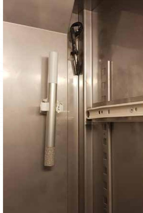
Senstick Microclimate installed inside the refrigeration unit.
